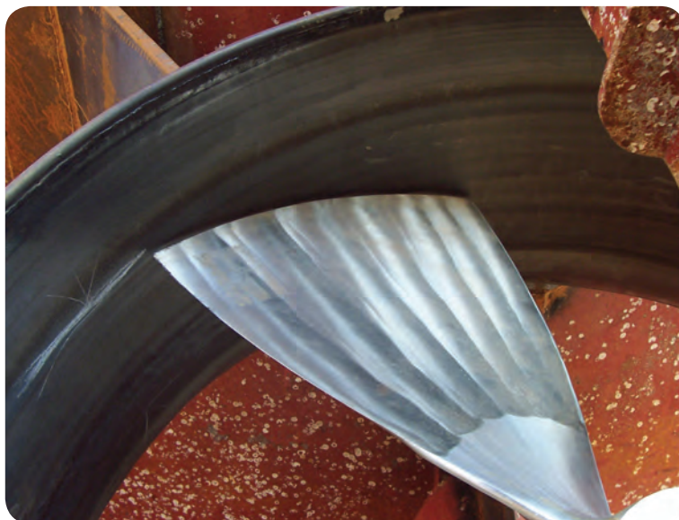
Figure 3. Coating Kort nozzle barrels with a thermally applied spray coating can eliminate the gap between the propeller blade tips and the wall of the Kort nozzle barrel, thereby making the nozzle more efficient.
