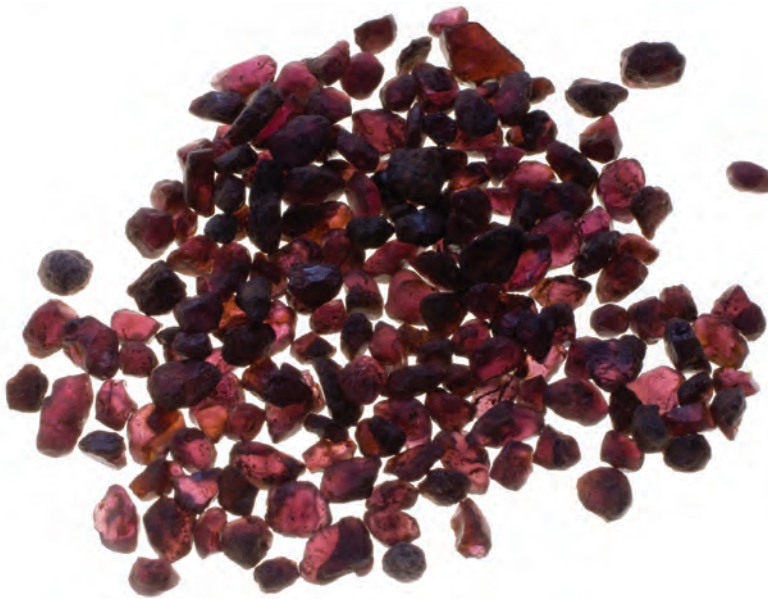
Garnet, a chemically inert and nonmetallic mineral, is probably the most used reclaimable abrasive.
