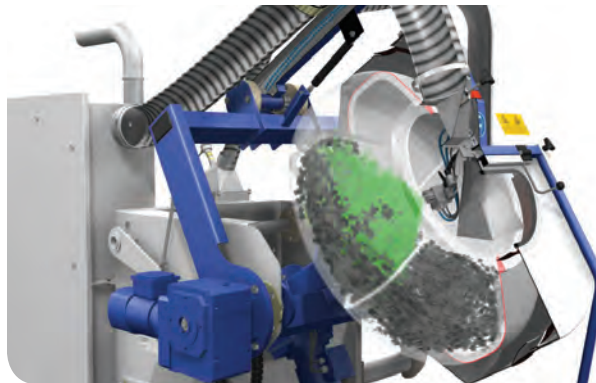
Figure 1. The system works by heating and tumbling small parts in an elliptical-shaped barrel beneath a spray nozzle or nozzles.
