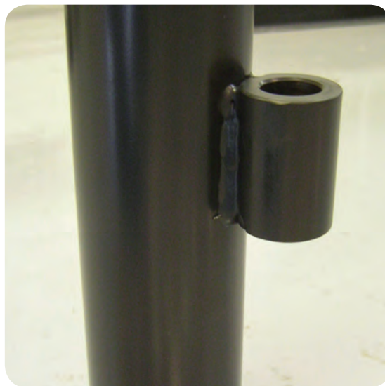
A 100% solids UV coating on a hydraulic cylinder. Photo courtesy of Strathmore Products, Inc.
