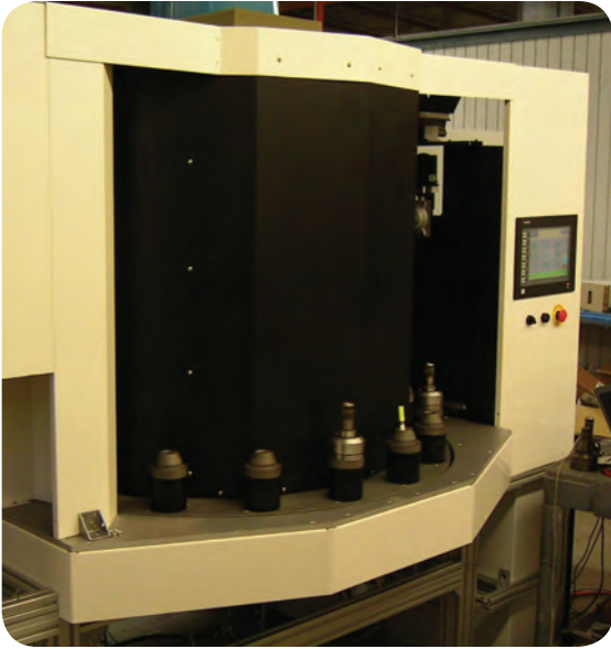
Figure 3. This four-walled finishing cell has self-contained spray application, air handling, liquid handling and UV curing. Image courtesy of Lesco – A Division of AUV.
