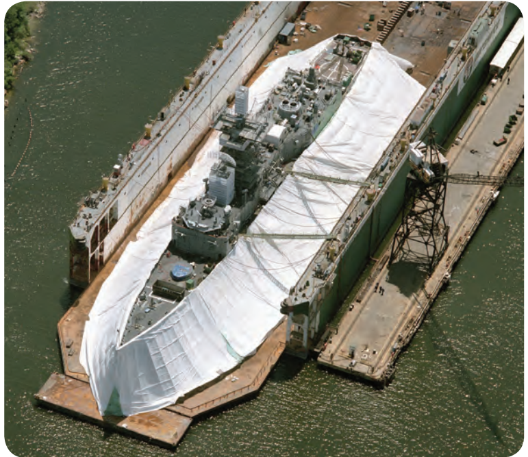
A ship in dry dock is blasted and painted under full containment. Photo courtesy of Eagle Industries.
