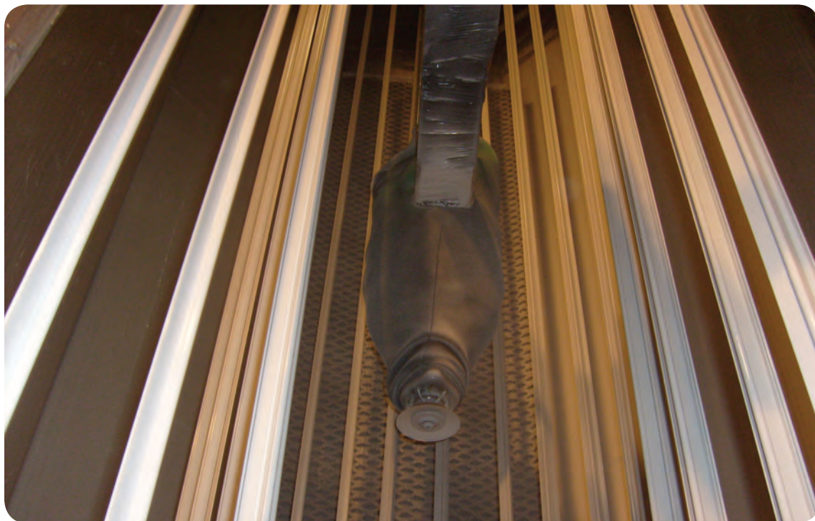
A typical aluminum extrusion application with a TurboDisk applicator.
