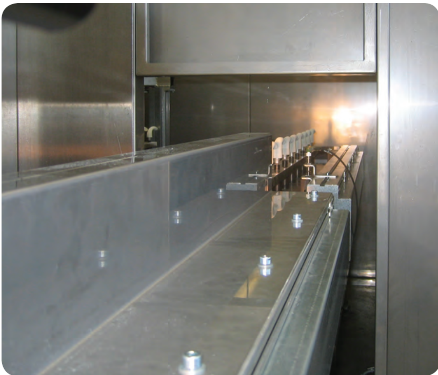
Figure 2. A fully automated production line with a line speed of 30 ft/min used for curing powder coatings on door handles.
