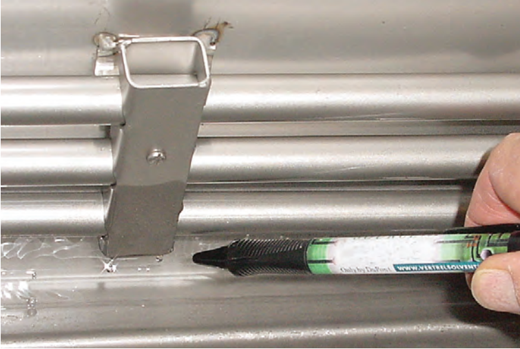
The primary condensing coils on a vapor degreaser, with droplets of solvent falling from the coils into the condensate trough in preparation for being recycled.
