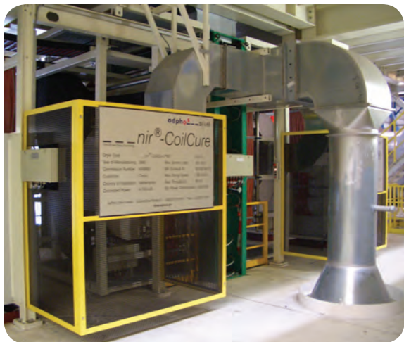
Figure 3. This in-line NIR system was recently placed in operation on the coil coating line of one of Europe's leading steel manufacturers.
