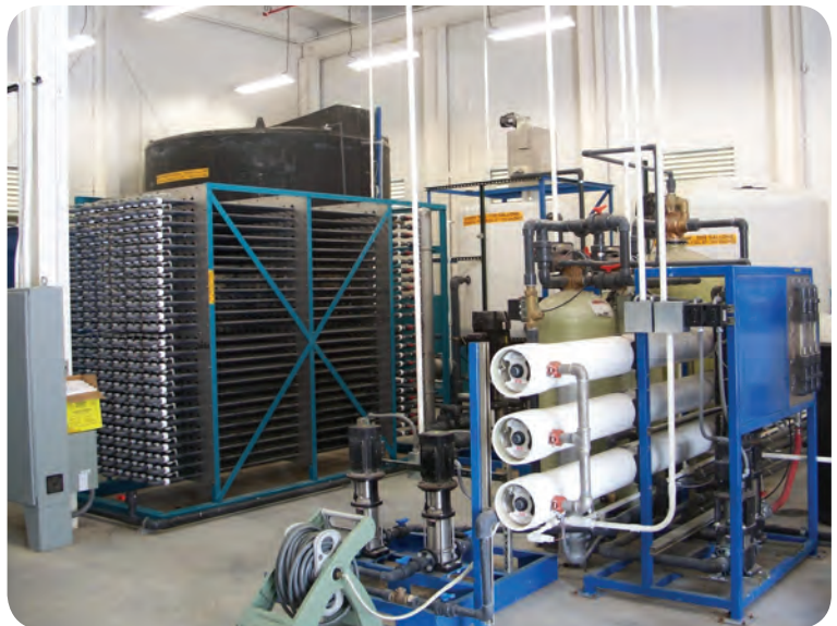
Ultrafiltration is used in the Reynosa plant to remove all suspended solids and oils effectively and to render the wastewater ready to be further processed for use in the plant. Photo courtesy of R3 Water Technologies.
