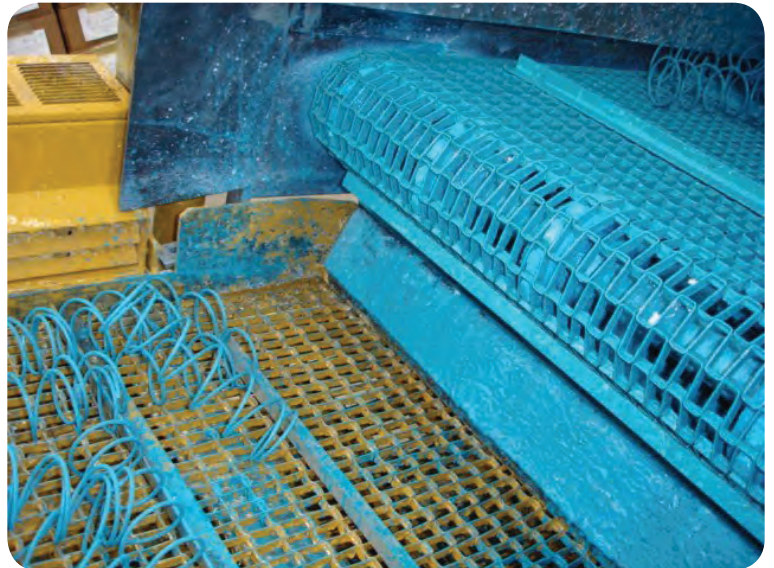
Water-based quench-coated springs entering a dryer oven.
