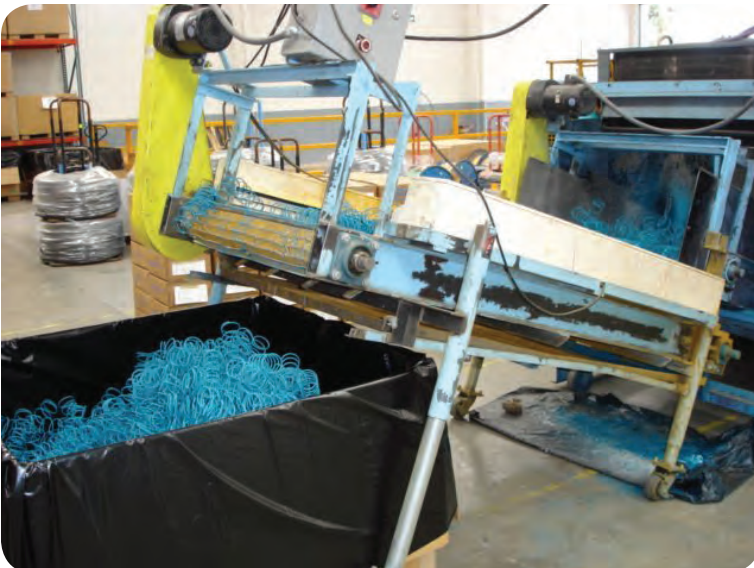
Water-based quench-coated springs exiting a dryer oven.
