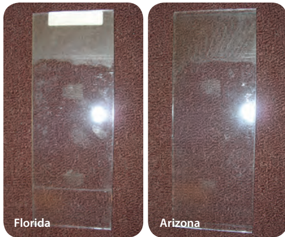
Figure 5. Photos of 5° weathering samples of polycarbonate coated with the new hardcoat system from Florida and Arizona testing. The top 20% of each panel was not coated and shows the effect of weathering exposure on uncoated PC. (Test results; actual results may vary.)
