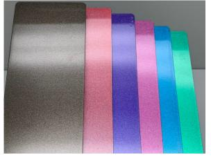
Aluminum pigment, organic pigments in combination with C-black in water borne metallic automotive coating. Excellent stabilization achieved using EDAPLAN 918 and LUBA-print 725.
