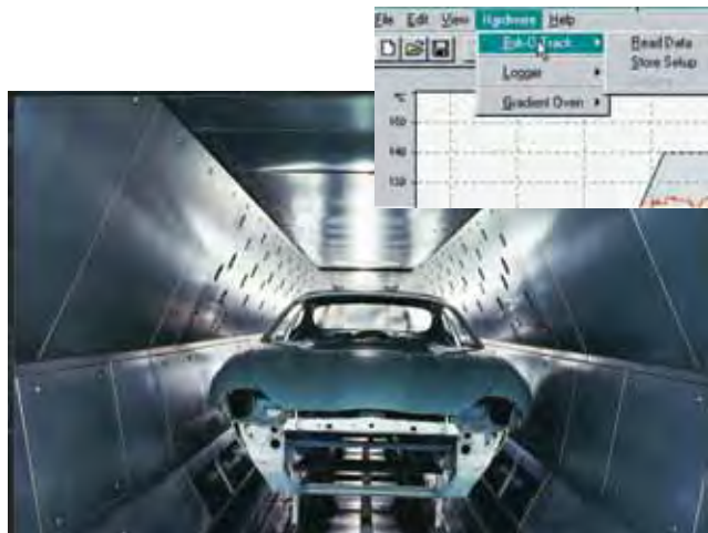
temp-gard collects temperature data in production oven.
