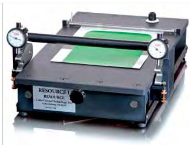
Resource I with bar type applicator and bar adapter
